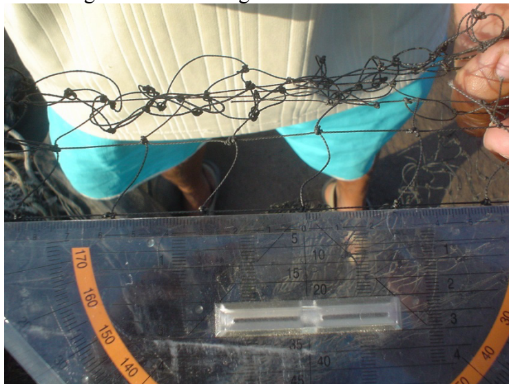
Figure C: Measuring the Fishnet Mesh Size
